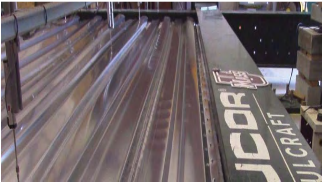
Figure 30: Typical end-warping behavior observed in the 36/4 specimens
